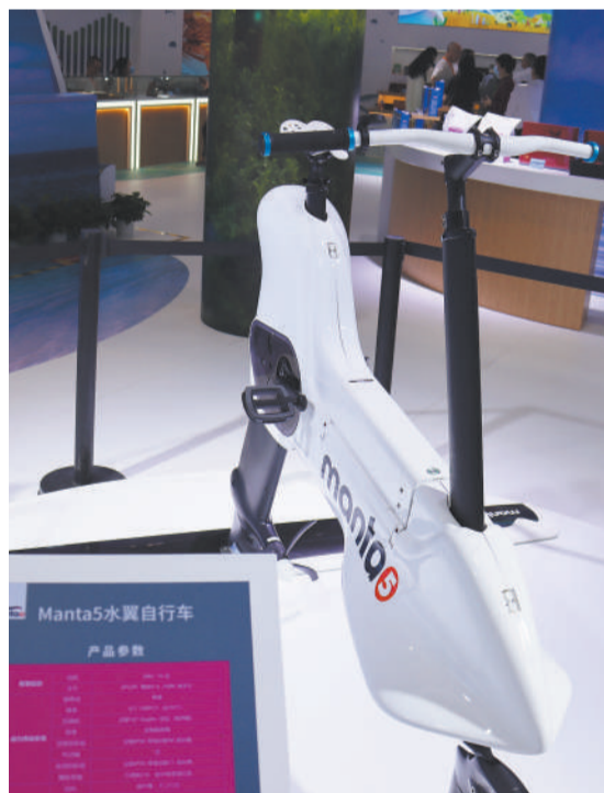
This hydrofoil e-bike made of carbon fiber can ride on water at a speed of 20 kilometers per hour.
