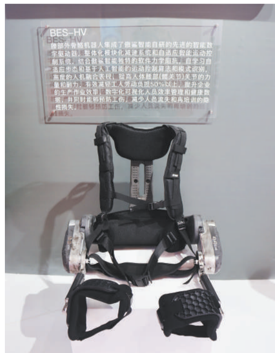
BES-HV waist exoskeleton robot can improve the strength and endurance of the waist and hip joint, which effectively reduces the labor burden of workers by more than 50 percent.
