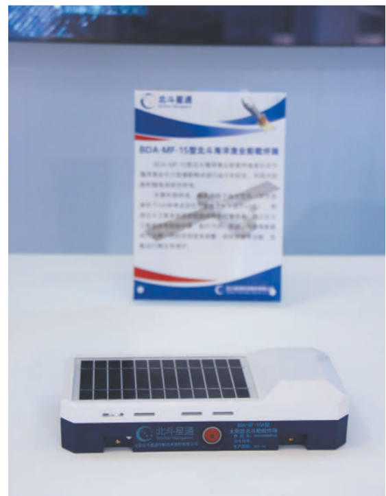
This marine fishery shipboard terminal is powered by a combination of solar energy and lithium batteries, using the Beidou Navigation Satellite System to locate ship positions.
