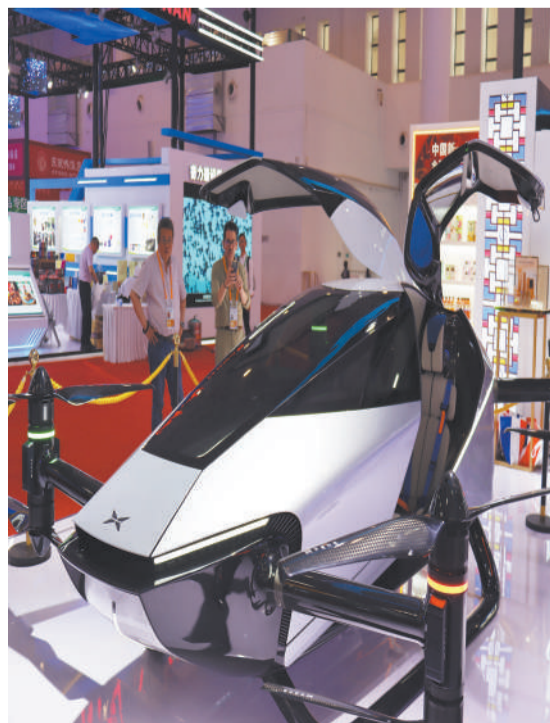
The XPENG X2 is a two-seater eVTOL flying car that can autonomously plan flight path and does not produce any carbon emissions during flight. (PHOTO: S&T DAILY/TANG ZHEXIAO/XINHUA)
