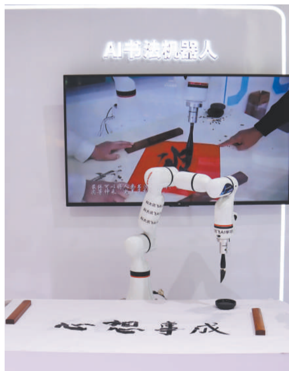
The AI robot arm with a Chinese calligraphy brush writes Chinese characters, which read "May all your wishes come true."
