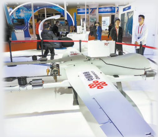
5G remote inspection unmanned aircraft system.
